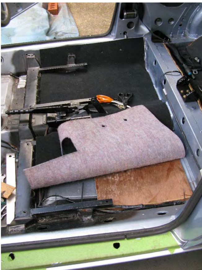
Trimming and fitting sound deadening material and plenty of waxoyl to keep the rust at bay. After final trimming the original carpet was refitted.
