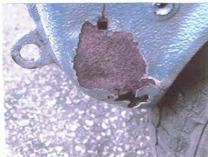
About that rust in the rear section of the wheel arch - it can't be that bad can it!
