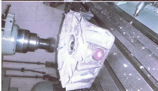
Roland has cut the SIMCA 1000 bellhousing back to accept the Honda Civic housing.
