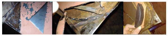
After completing the repairs on both back doors I commenced work on one of my original front doors. I replaced the bottom corners and the door was looking a million dollars until I decided to tackle a couple of small rust spots on the face of the door.
