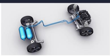
With Hybrid Air Technology, the PSA Group who put this article out combines the environmental advantages of compressed air and the performance of a petrol engine without using electricity.
